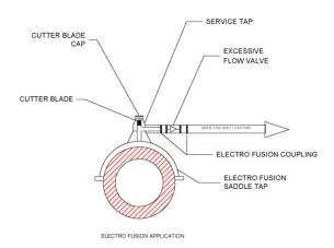
All polyethylene main taps on the City of Port Aransas Natural Gas System shall be an Electro-Fusion Saddle Tap w/Butt-Fusion Outlet.
