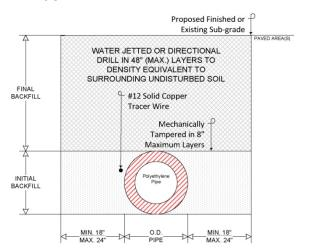
Backfill in layers of two inch (2") – four inch (4") clean sand, embedding to the top crown of the pipe and mechanically tamper to a density equivalent of not less than 100% of an ASTM D698 Proctor Curve. Native soils may be used provided that the embedment material soil type and particle size is in accordance with ASTM D 2774. Embedment shall be placed and compacted to at least 90% Standard Proctor Density in six inch (6") lifts
