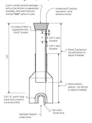
Valve supports shall be installed for all one inch (1") thru four inch (4") polyethylene valves.
