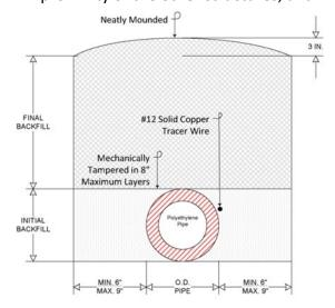
to allow the required space for future maintenance or repairs of the newly installed Gas distribution pipe. This alternative shall *necessitate approval* by the City of Port Aransas Gas Department.
